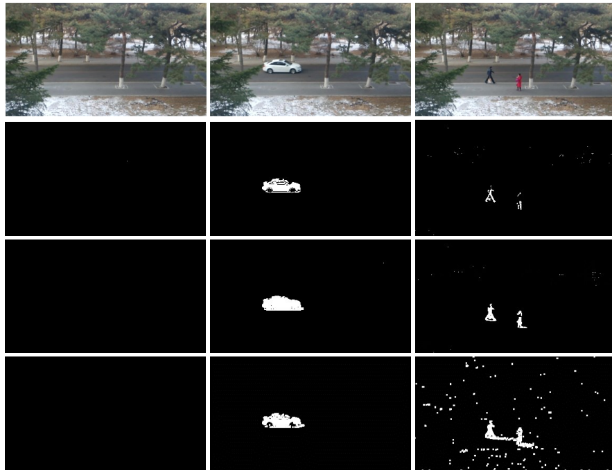
Fig. 9 Result images by initial and improved ViBe algorithm: 1 th row - Original frame; 2 th row - Initial ViBe; 3 th row – Improved ViBe; 4 th row – GMM
