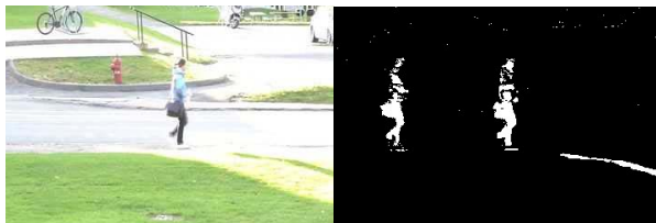
Fig. 2 The ghost appearance in the motion detection result by using of ViBe algorithm.
