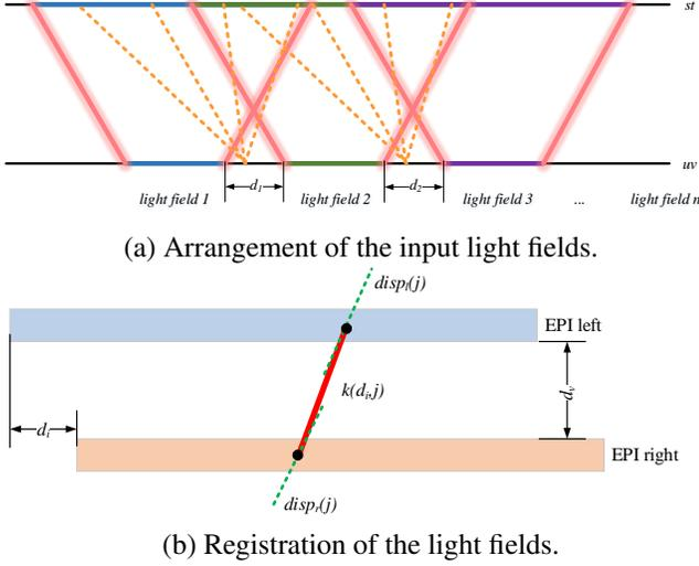
**Fig. 3.** (a) Totally  $n$  light fields are represented on the common two-plane  $uv - st$ . The pink lines are light rays captured by the camera and the orange ones are missing rays. (b) The blue EPI is from the left light field and the orange one is from right. Vertical distance between two EPIs  $d_v$  is relative to  $d_i$ .  $disp_l(j)$  and  $disp_r(j)$  (green lines) are coherent with geometry slope  $k(d_i, j)$  (red line).
